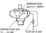
An additional G<sup>1</sup>/4" (BSPF) drain port in the front mounting flange is provided when the "V" (shaft vertically upwards) designator is given after the shaft type letter in position **3** of the model code. This additional drain should be connected into the main motor casing drain line downstream of a 0,35 bar (5 psi) check valve to ensure lubrication of the upper bearing, see above diagram.
