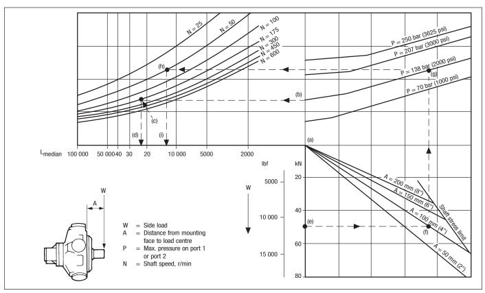
The nomograph allows the median▲ bearing life to be determined for conditions of:
