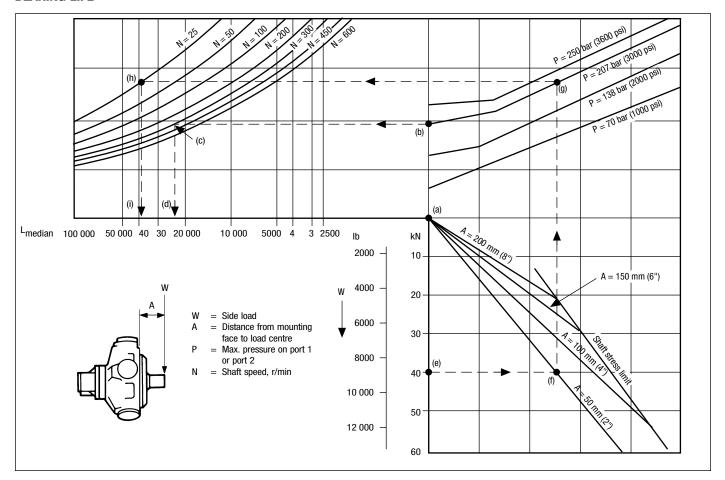
The nomograph allows the median **bearing** life to be determined for conditions of:
