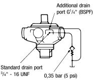
An additional G¹/4" (BSPF) drain port in the front mounting flange is provided when the "V" (shaft vertically upwards) designator is given after the shaft type letter in position 3 of the model code. This additional drain should be connected into the main motor casing drain line downstream of a 0,35 bar (5 psi) check valve to ensure lubrication of the upper bearing. See above diagram.
