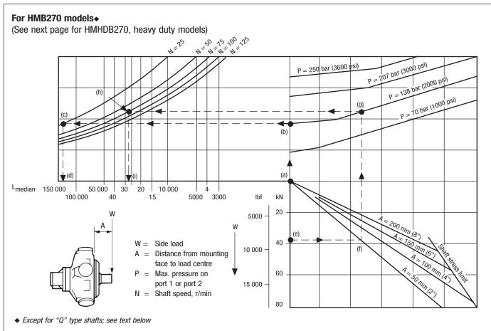
The nomographs on this and the following page allow the median▲ bearing life to be determined for conditions of:
