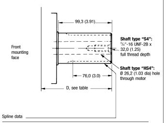
For shaft types "S4" and "HS4" Involute gear tooth form
