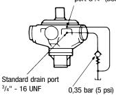
An additional G¹/₄" (BSPF) drain port is provided when the "V" (shaft vertically upwards) designator is given after the shaft type letter in position of the model code. This additional drain should be connected into the main motor casing drain line downstream of a 0,35 bar (5 psi) check valve to ensure lubrication of the upper bearing, see above diagram.
