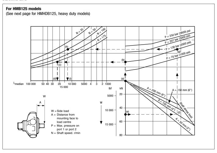
The nomographs on this and the following page allow the median bearing life to be determined for conditions of:
