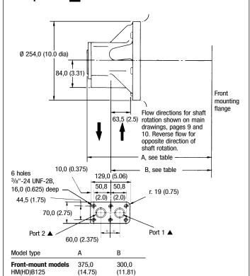
▲ Ø 28 (1.125 dia), with recess for 31,0 (1.22) i/d x Ø 4 (0.157 dia) section 0-ring
