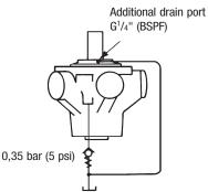
An additional G<sup>1</sup>/4" (BSPF) drain port is provided when the "V" (shaft vertically upwards) designator is given after the shaft type letter in position 3 of the model code. This additional drain should be connected into the main motor casing drain line downstream of a 0,35 bar (5 psi) check valve to ensure lubrication of the upper bearing, see above diagram.
