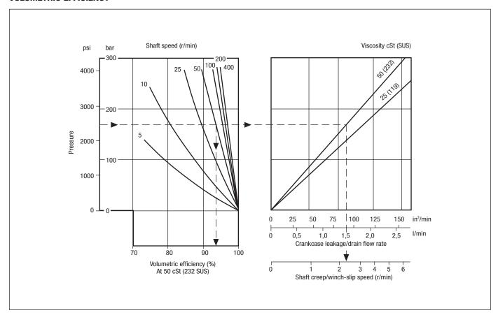
This nomograph enables the average volumetric efficiency, crankcase (drain) leakage and "winch slip"/shaft creep speed to be estimated.
